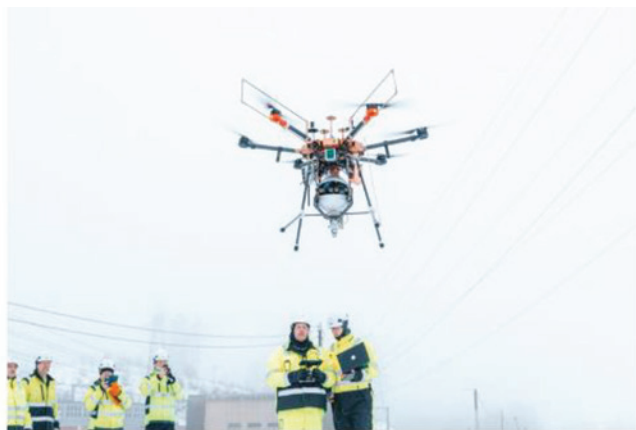
Heimdall Power uses autonomous drone installation technology to place its Neuron sensors on live transmission lines.
