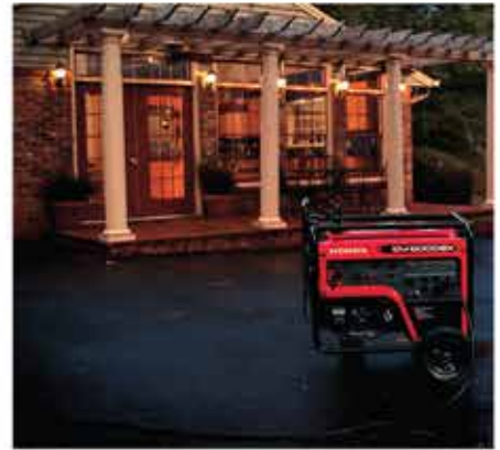
Position portable generators at least 25 feet outside the home, away from doors, windows and vents that can allow CO to enter the home. (Photo Source: Honda)
