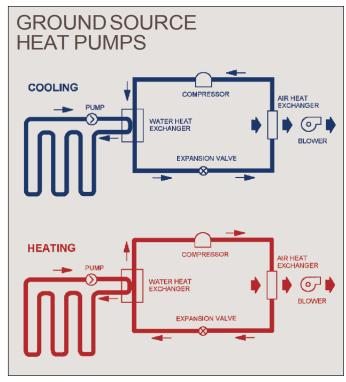
Ground source heat pumps use the earth's ability to store heat in the ground.
