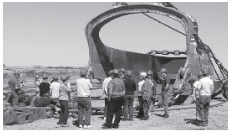
Participants in Steele-Waseca's 2016 Coal Creek Tour had the opportunity to get a close-up view of the drag line that uncovers the lignite coal at Falkirk Mine used for electrical production at the power plant.
