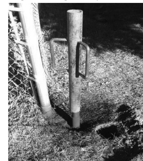
Minnesota Rural Electric Association (MREA) Safety Playbook reported an electric co-op member had attempted to locate a wire and believed they were in the clear when they attempted to drive in a post only to strike a primary wire. The fault went back to the 3-phase recloser at the substation. The fault burnt the post and grass around it. The member called 911 and fortunately wasn't injured. He was very lucky that he wasn't hurt or killed and was encouraged to have wires located before driving in any more fence posts. (Courtesy MREA Safety Playbook - Oct. 2, 2015)
